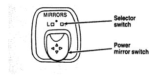
The electric remote control mirror switch
