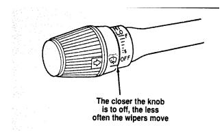
The windshield wiper on the turn signal lever
