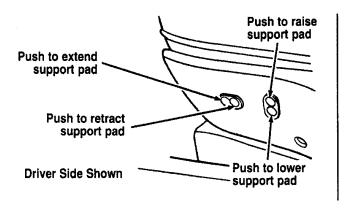
The seat controls for the lumbar support on the driver's seat
