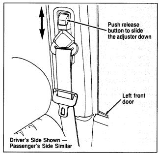
Figure I - The shoulder belt height adjuster
