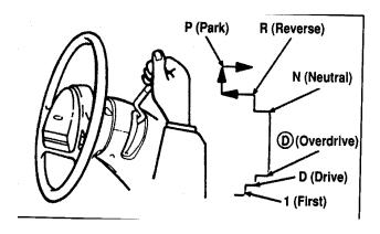
The positions of the column-mounted gearshift
