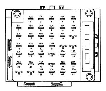
The instrument panel fuse panel
