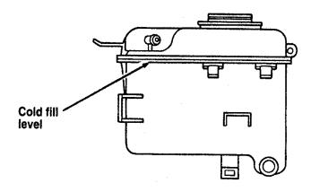
The engine coolant reservoir
