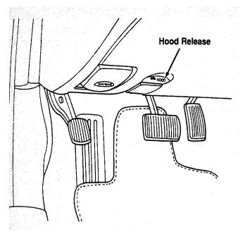
The hood release under the instrument panel
