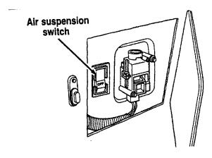
The air suspension switch - located in the trunk
