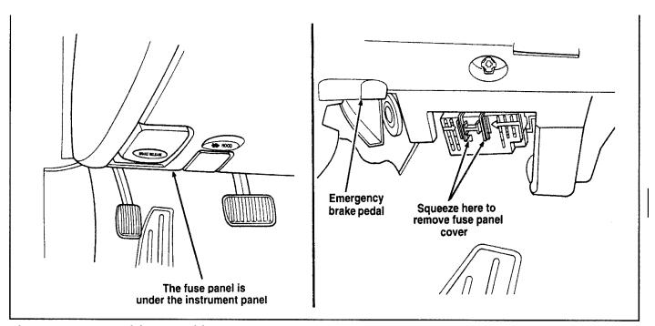
The instrument panel fuse panel location
