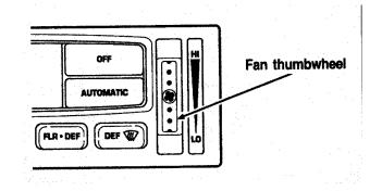
When you move the thumbwheel, the fan speed will go to manual control. The display window will show the symbol in the lower right corner along with the selected temperature and operating function.
