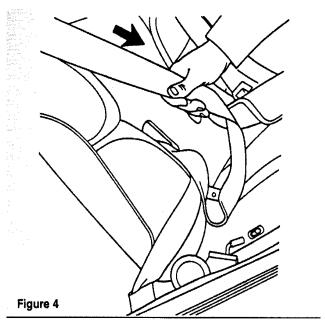
Setting the retractor to automatic locking mode
