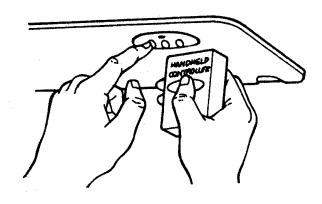
4. When the Universal Transmitter light begins to flash rapidly (this could take up to 60 seconds), release both buttons. You can now use your Universal Transmitter instead of the hand-held controller.
