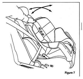
Checking that the seat is secure
