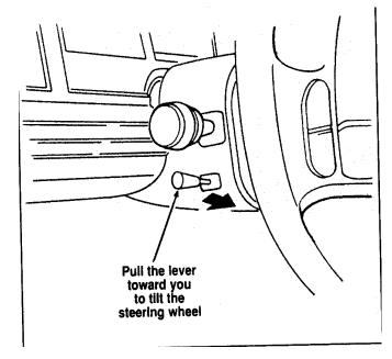
The lever to tilt the steering wheel
