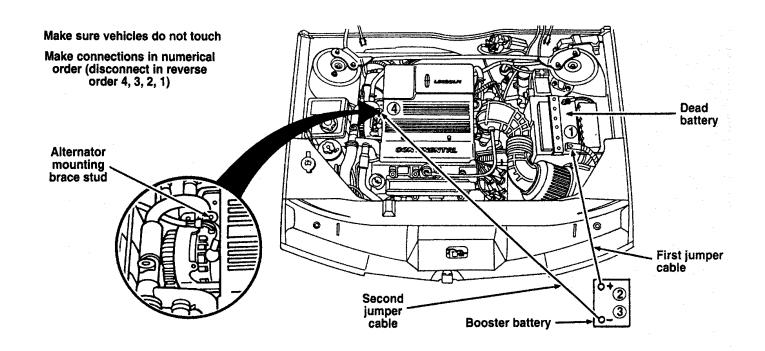
The engine with jumper cables
