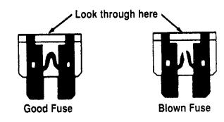
The side view of a Blade type fuse
