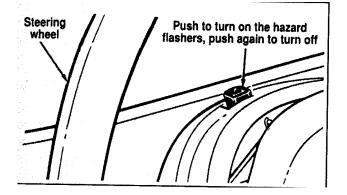
The control switch for hazard flashers
