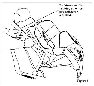
Checking that retractor is in automatic locking mode
