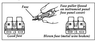
Fuse puller tool and fuse
