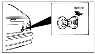
Unlocking the hatchback lid with the key
