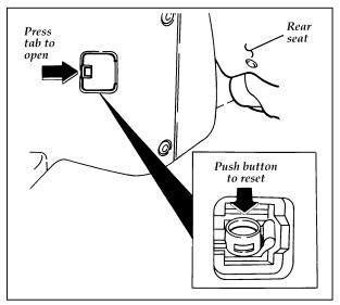
The location of the fuel pump shut-off switch (U.S. vehicle shown — Canadian vehicles similar)
