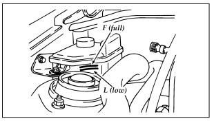
Where to check the power steering fluid
