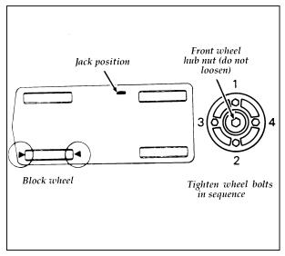
Blocking the wheel diagonally opposite the tire being changed
