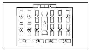
Fuse panel in the instrument panel
