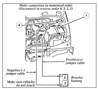
The sequence for connecting the jumper cables
