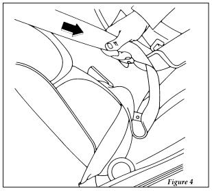
Setting the retractor to automatic locking mode
