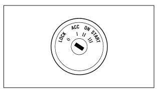
Ignition lock cylinder (automatic transaxle)
