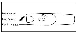
High beam and flash-to-pass operation
