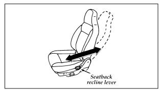
The lever used to recline the back of the seat
