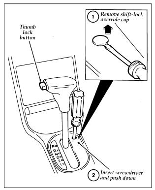
Operating the shift-lock override mechanism
