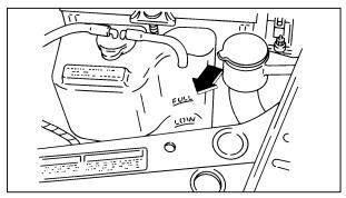
Engine coolant recovery reservoir
