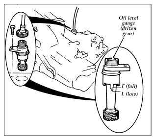
Checking manual transaxle oil level
