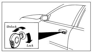
Using the key to lock or unlock the front door
