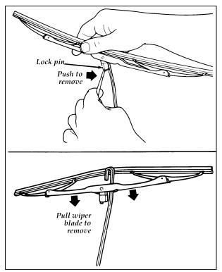
Replacing the wiper blades
