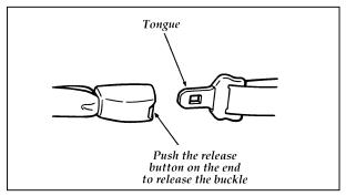
Unfastening the combination lap/shoulder belts — front and rear outboard seating positions
