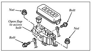
**Removing fuse block**
