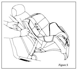
Checking that the seat is secure
