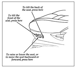
The power controls on the driver's seat
