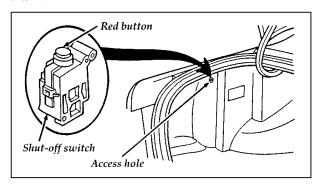
The fuel pump shut-off switch
