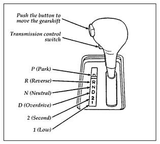
The positions of the console-mounted gearshift
