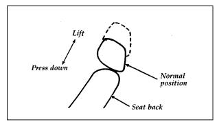
Adjusting the head restraint
