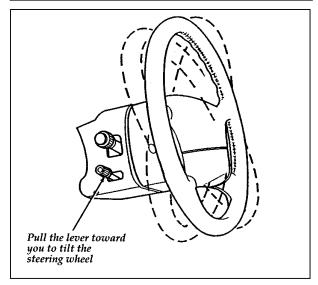
The lever to tilt the steering wheel
