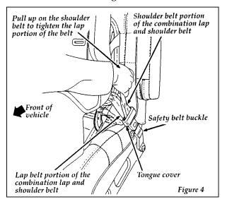
7. Grasp belt close to child seat and pull on the shoulder belt portion of the combination lap/shoulder belt, then allow the belt to retract and remove all slack to securely tighten the child safety seat in the vehicle. See Figure 5.
