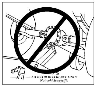
The improper lift point
