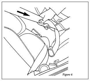
Setting the retractor to automatic locking mode
