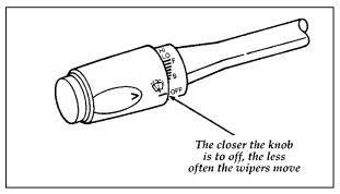
The variable interval wiper on the turn signal lever To set the interval wipers, turn the knob at the end of the turn signal lever toward or away from you until the wipers are going at the desired interval.
