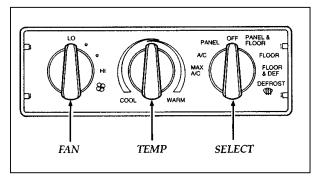
The controls for the manual heating and air conditioning system
