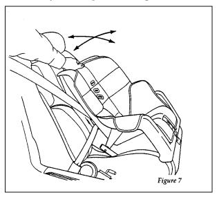
Checking that the seat is secure
