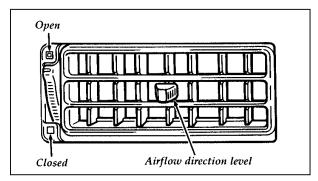
Controlling the airflow from panel registers
