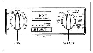
The controls for the Semi-Automatic Temperature Control system
