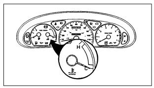
The engine coolant temperature gauge
