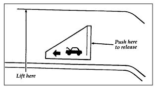
The auxiliary catch under the front edge of the hood
