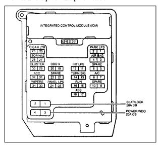
The instrument panel fuse panel
