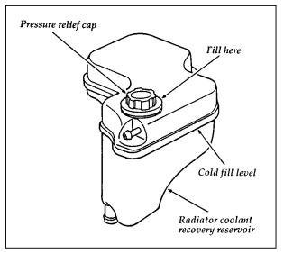
The engine coolant reservoir
