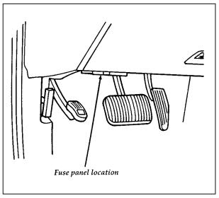
The instrument panel fuse panel location
