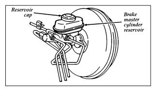
The brake system fluid reservoir
