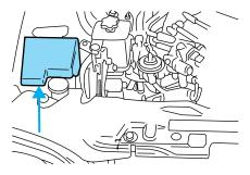
Always disconnect the battery before servicing high current fuses.
