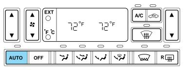
Press and hold the AUTO control for about two seconds to equalize the passenger set temperature with the driver side temperature. This feature is useful when the driver is alone in the vehicle.
