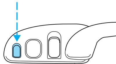
With the ignition key in the ACC or ON position, the reading lamp can be turned on by pressing the rocker control.
