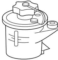
5. If the fluid is low, add fluid in small amounts, continuously checking the level until it reaches the range between the MIN and MAX lines. Be sure to put the cap back on the reservoir.
