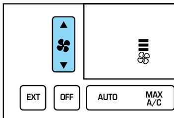
The display will show
