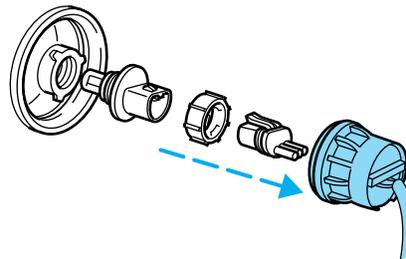
5. Disconnect the electrical connector from the bulb by pulling rearward.
