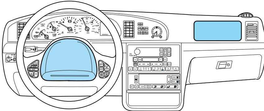
Your vehicle is equipped with a crash sensing and diagnostic module which records information about the air bag and sensor systems. In the event of a collision this module may save information related to the collision including information about the air bag system and impact severity. This information will assist Ford Motor Company in servicing the vehicle and in helping to better understand real world collisions and further improve the safety of future vehicles.
