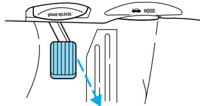
The BRAKE warning lamp in the instrument cluster illuminates and remains illuminated (when the ignition is turned ON) until the parking brake is fully released.
