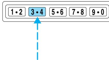
To release the trunk, enter the factory-set code or personal code (driver door unlocks) and press 5/6 within 7.5 seconds.
