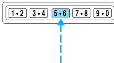
After the factory-set code or personal code has been entered, you can unlock all doors (press 3/4) and release the trunk (press 5/6) as long as the controls are pressed within 7.5 seconds of each other.
