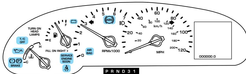
Make sure the corresponding lights illuminate or illuminate briefly. If a light fails to illuminate, have the vehicle serviced.
