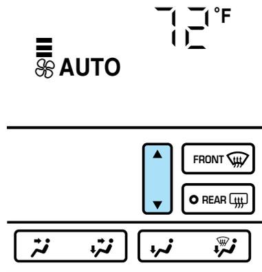
For continuous maximum cooling, push the temperature control until 16°C (60°F) is shown in the display window. The EATC will continue maximum cooling (disregarding the displayed temperature) until a warmer temperature is selected by pressing the temperature control.
