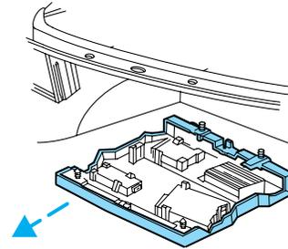
5. Carefully remove the bulb socket from the lamp assembly.
