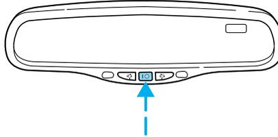
The mirror will automatically return to the normal state whenever the vehicle is placed in R (reverse)(when the mirror is on) to ensure a bright clear view when backing up.
