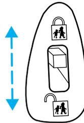
Move lock control up to engage the childproof lock. Move control down to disengage childproof locks.
