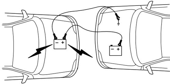
4. Make the final connection of the negative (-) cable to an exposed metal part of the stalled vehicle's engine, away from the battery and the carburetor/fuel injection system. **Do not** use fuel lines, engine rocker covers or the intake manifold as *grounding* points.
