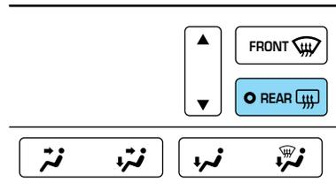
The ignition must be in the ON position to operate the rear window defroster.
