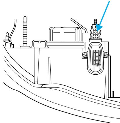
3. Use a 4 mm wrench or socket to turn the horizontal adjusting screw until the "0" mark on the yellow dial lines up with the reference mark on the marker (as shown) when viewed directly from above.
