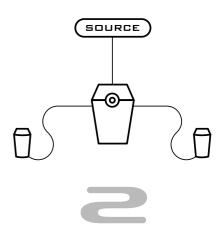
Comprises an active sub woofer with system volume control plus two satellites.
