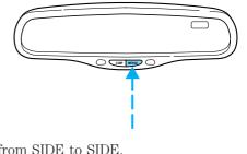
Press the control to turn the mirror on or off.
