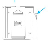
4. Insert one disc into each CD tray of the magazine (up to 6 discs). Ensure that the label side is facing up.
