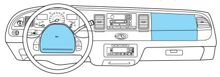
Your vehicle is equipped with a crash sensing and diagnostic module which records information about the air bag and sensor systems. In the event of a collision this module may save information related to the collision including information about the air bag system and impact severity. This information will assist Ford Motor Company in the servicing vehicle and helping to better understand real world collisions and further improve the safety of future vehicles.
