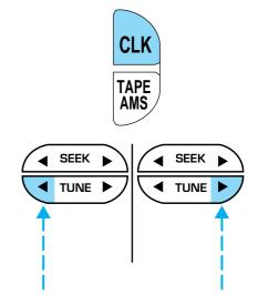
The CLK control will allow you to switch between media display mode (radio station, stereo information, etc.) and clock display mode (time). When in clock mode, the media information will display for 10 seconds, when the radio is turned on, and then revert to clock information. Any time that the media is changed, (new radio station, etc.), the media information will again display for 10 seconds before reverting back to the clock. In media mode, the media information will always be displayed.
