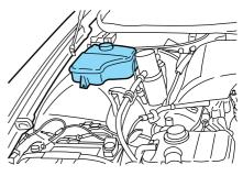
State or local regulations on volatile organic compounds may restrict the use of methanol, a common windshield washer antifreeze additive. Washer fluids containing non-methanol antifreeze agents should be used only if they provide cold weather protection without damaging the vehicle's paint finish, wiper blades or washer system.
