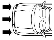
cause activation. Front air bags are designed to inflate in frontal and near-frontal collisions, not rollover, side-impact, or rear-impacts unless the collision causes sufficient longitudinal deceleration.
