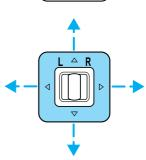
3. Return to the center position to lock mirrors in place.
