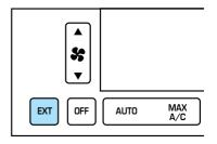
If a manual override function is selected while the outside temperature is displayed, the new function will be displayed for four seconds after it is changed, then the outside temperature will return to the window along with the override selection.
