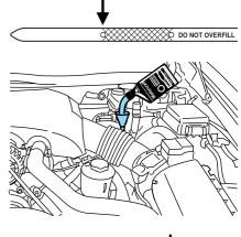
• Do not overfill the engine with oil. Oil levels above this mark may cause engine damage. If the engine is
