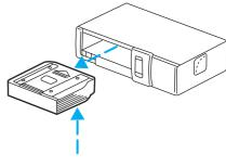
3. Pull the lever to remove a CD tray from the magazine.
