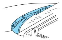
• Do not place objects over the defroster outlets. These objects can block airflow and reduce your ability to see through your windshield. Avoid placing small objects on top of the instrument panel. These objects may fall down into the defroster outlets and block airflow, in addition to damaging the climate control system.
