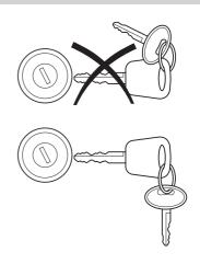
key ring held away from the ignition key. Check to make sure the **coded** key is an approved Ford **coded key**.
