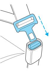
5. To put the retractor in the automatic locking mode, grasp the shoulder portion of the belt and pull downward until all of the belt is extracted and a click is heard.
