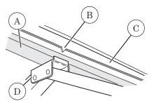
Position the jack according to the following guides and turn the jack handle clockwise until the wheel is completely off the ground.
