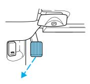
The BRAKE warning lamp in the instrument cluster illuminates and remains illuminated (when the ignition is turned ON) until the parking brake is fully released.
