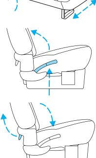
Pull control up to flip seatback to forward flat position.
