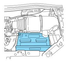
However, for severe usage or in high temperature climates, check the battery electrolyte level. Refer to the scheduled maintenance guide for the service interval schedules.
