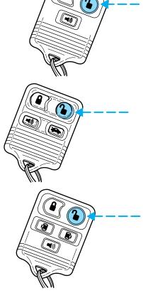
Press this control to unlock the driver door and disarm the anti-theft system (if equipped). The interior lamps will illuminate.
