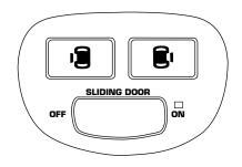
With this option, you can open and close the sliding door(s) with the controls inside your vehicle. With the remote keyless entry system, you can also operate the PSD with the remote transmitter. Refer to *Remote Entry System* in this chapter.
