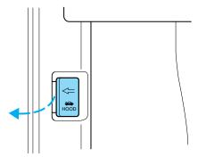
2. Go to the front of the vehicle and release the auxiliary latch that is located under the front center of the hood.
