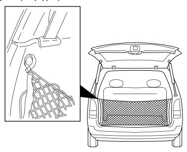
The cargo net secures lightweight objects in the cargo area. Attach the net to the anchors provided. Do not put more than 22 kg (50 lbs.) in the net. This net is not designed to restrain objects during a collision.
