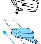
4. While holding the shoulder and lap portions together, route the tongue and webbing through the child seat according to the child seat manufacturer's instructions. Be sure that the belt webbing is not twisted.
