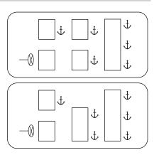
The tether can be attached directly to the rear of all passenger seating except the front passenger seat equipped with power adjustment. The front passenger seat with manual adjustment does have a tether anchor.
