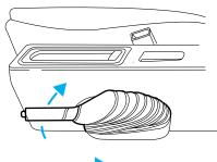
5. Turn the key to 4 (ON) without turning the key to 5 (START).
