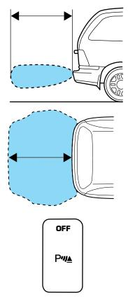
The OFF indicator remains illuminated when the system is disabled. The system defaults to ON every time the reverse gear is selected. Press the control to disable or enable the system.
