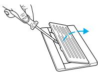
• To install the tub cover(s), first insert the tabs located on the opposite side of the pry location into the slots of the floor tub then press down on the other side of the cover until it snaps into place securely. (Additional tub covers can be purchased as an accessory from your dealer.)
