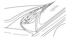
• Do not place objects over the defroster outlets. These objects can block airflow and reduce your ability to see through your windshield. Avoid placing small objects on top of the instrument panel. These objects may fall down into the defroster outlets and block airflow, in addition to damaging the climate control system.
