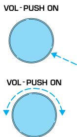
If the volume is set above a certain level and the ignition is turned off, the volume will come back on at a "nominal" listening level when the ignition switch is turned back on.
