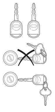
**coded key** ignition key, but can cause a momentary issue if they are too close to the key during engine start. If a problem occurs, turn ignition OFF and restart the engine with all other objects on the key ring held away from the ignition key. Check to make sure the **coded key** ignition key is an approved Ford **coded key** ignition key.
