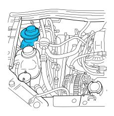
5. If the fluid is low, add fluid in small amounts, continuously checking the level until it reaches the correct operating range. Be sure to put the cap back on the reservoir.
