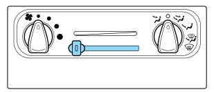
Controls the temperature of the airflow inside the vehicle.
