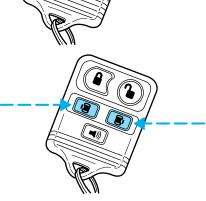
Press this control twice within three seconds to open the power sliding door (if equipped). The interior lamps will illuminate. Press this control another two times within three seconds to close the power sliding door and turn off the interior lights.
