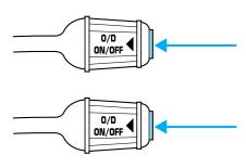
When you shut off and re-start your vehicle, the transaxle will automatically return to normal ( Overdrive) mode.
