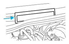
4. Lift and remove the cabin air filter.
