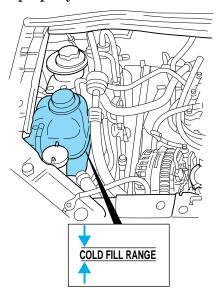
The engine coolant should be at the "cold fill level" or within the "cold fill range" as listed on the engine coolant reservoir (depending upon application).
