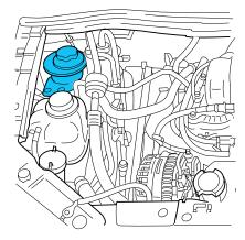
Check the power steering fluid. Refer to the scheduled maintenance guide for the service interval schedules. If adding fluid is necessary, use only MERCON® ATF.
