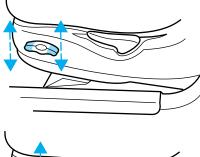
Press control to raise or lower the seat, or to move the seat forward or backward.
