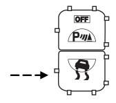
cluster that will illuminate when the system is active. If a failure is detected, the "TRAC OFF" indicator light will stay ON, vehicles with a message center (if equipped) will also display the warning "CHECK ADVANCETRAC", have the system serviced immediately.
