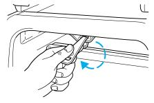
8. Tighten the child safety seat tether strap according to the manufacturer's instructions.
