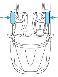
Side air bags, in combination with seat belts, can help reduce the risk of severe injuries in the event of a significant side impact collision.
