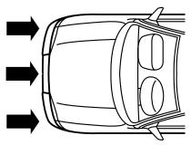
cause activation. Front air bags are designed to inflate in frontal and near-frontal collisions, not rollover, side-impact, or rear-impacts unless the collision causes sufficient longitudinal deceleration.
