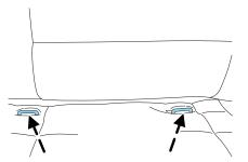
Attach the lower anchors for child seat installation or lower anchors for child seat installation-compatible child seat only to the appropriate locations shown.
