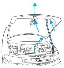
3. Lift the hood and secure it with the prop rod. Your vehicle's hood has two locations for the prop rod to be placed. These locations provide two different hood opening positions. Use the location which best suits your needs.
