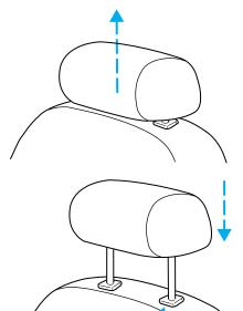
Push control to lower head restraint.
