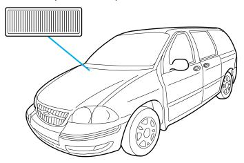
The cabin air filter restricts the entry of airborne dust and pollen particles. The filter is located just in front of the windshield under the cowl vent screen on the passenger side of the vehicle.
