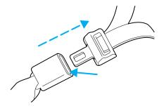
The front and rear outboard safety restraints in the vehicle are combination lap and shoulder belts. The front and rear seat passenger outboard safety belts have locking cinch tongues described below:
