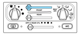
Controls the temperature of the airflow for the front part of the passenger compartment.
