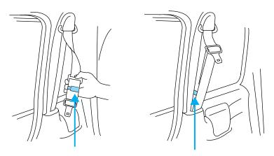
2. (For 2nd row bench seat only.) Using the clip attached to the end of the shoulder belt(s), clip the end of the belt to the stationary portion of the shoulder belt coming out of the trim panel. The end of the shoulder belt **must** be clipped in order to keep it from striking anything during vehicle operation.
