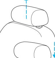
Push control to lower head restraint.
